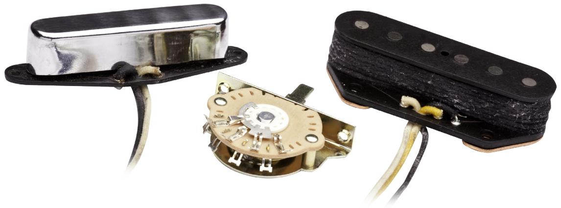
This set combines Seymour's favorite Tele<sup>®</sup> pickup—the '53 Style Tapped Tele<sup>®</sup> Lead—in his favorite combination Custom Wound Telecaster<sup>®</sup> Rhythm pickup. The rhythm pickup is reverse wound with reverse polarity, in order to offer hum-canceling when both pickups are on.
